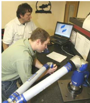
Billy Pederson & Jeff Bontrager, take critical measurements of a part with the new Faro Arm purchased this fall.
